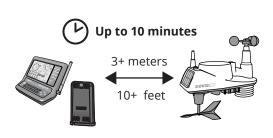
Verify data transmission from the Sensor Suite to the WeatherLink app and/or to the Console.
