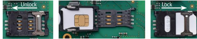
1. Slide the metal part of the SIM card holder to unlock it.
